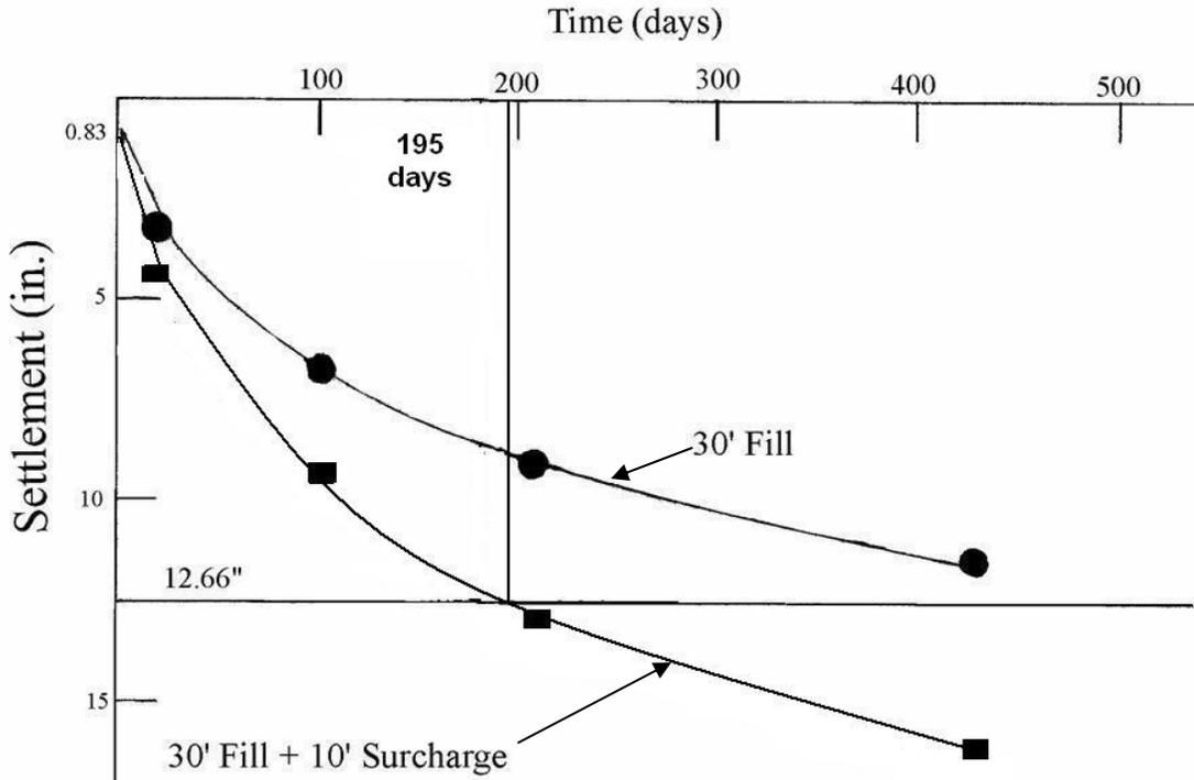
**Figure A.6-8. Settlement vs. Time after construction of 30 ft embankment fill with and without surcharge.**
