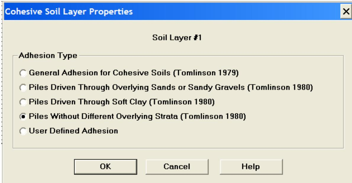
Figure 9-23. DRIVEN Cohesive Soil Layer Properties screen.
