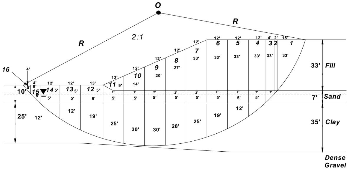
Figure A.5-4. Vertical slices above assumed failure arc – East Abutment.
