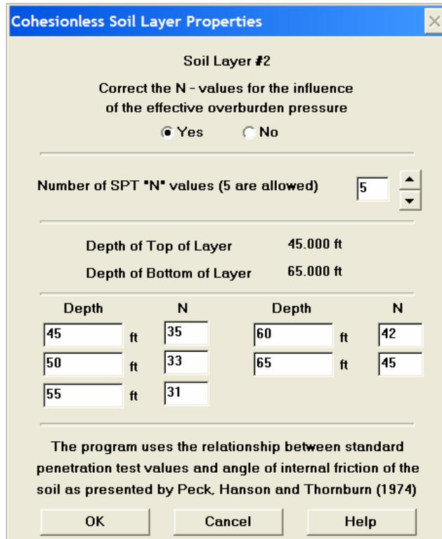
Figure 9-25. DRIVEN Cohesionless Soil Layer Properties screen.
