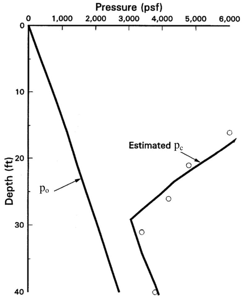
Figure A.4-4. Plot of estimated preconsolidation pressure,  $p_c$ , on a  $p_o$  plot.
