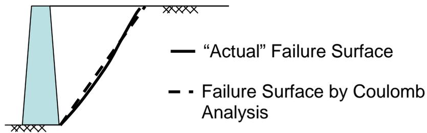
(a) Active Case ( $\phi' = 30^\circ$ ,  $\delta = 30^\circ$ )
