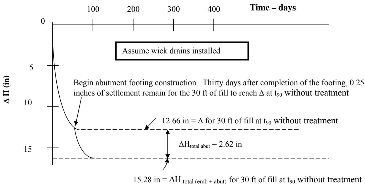
**Figure A.7-8. Settlement –Time curve for abutment footing built 6 months after completion of embankment fill with vertical drain pre-treatment.**
