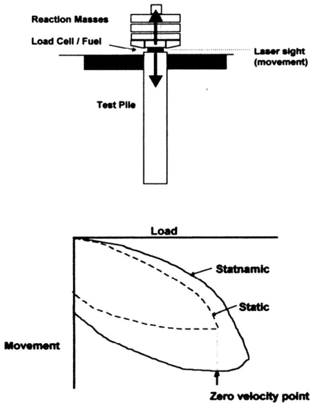
Figure 9-76. Schematic of Statnamic<sup>®</sup> test
