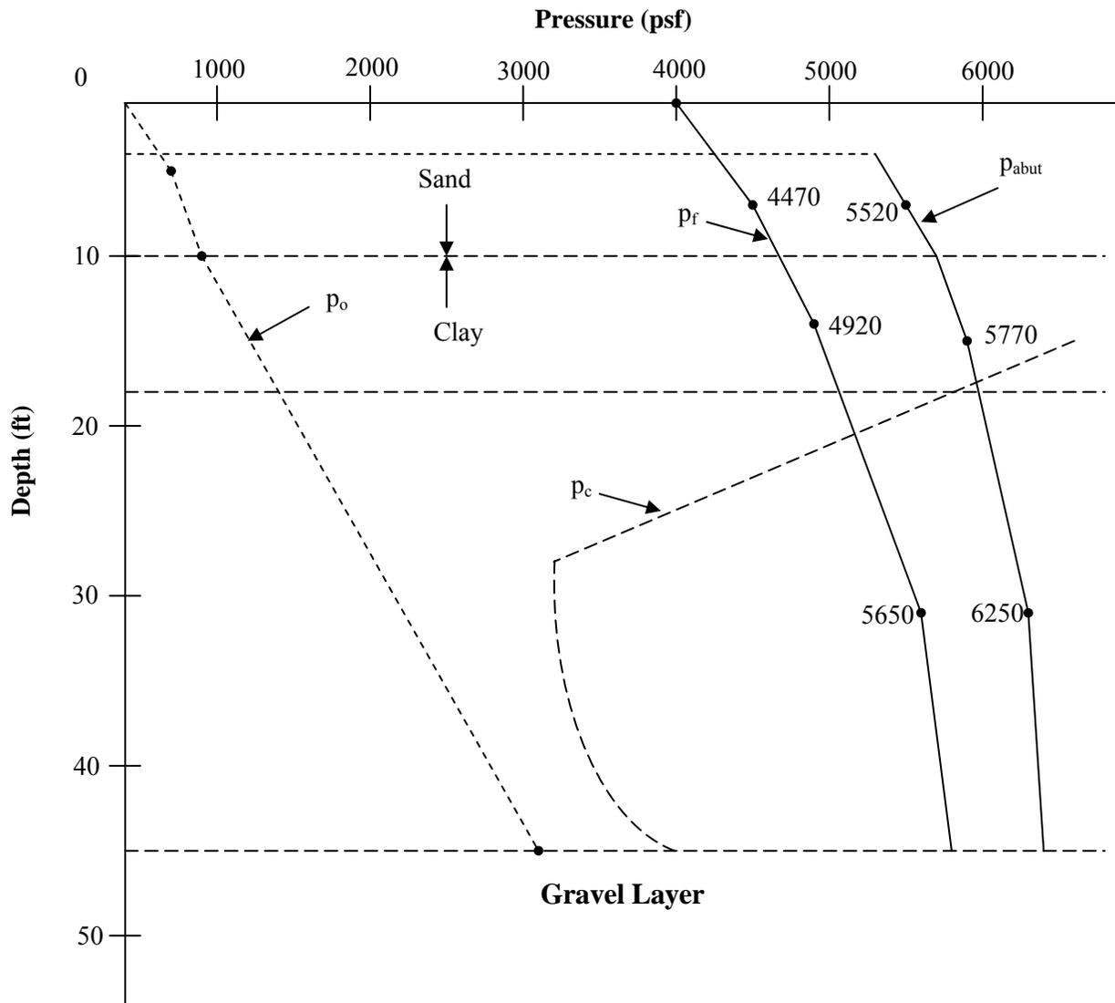
**Figure A.7-6. Pressure distributions with depth at East Abutment for the overburden pressure ( $p_o$ ), preconsolidation pressure ( $p_c$ ), final pressure due to embankment fill only ( $p_f$ ), and the final pressure due to embankment fill plus abutment footing ( $p_{abut}$ ).**
