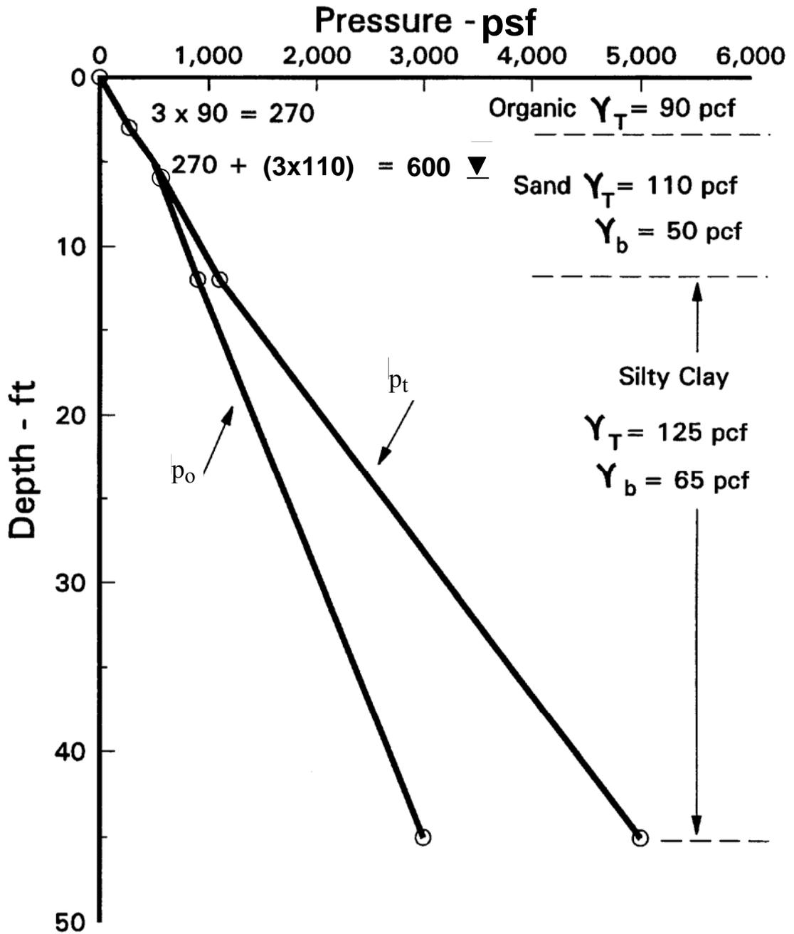
Figure A.4-2. The  $p_o$  diagram for boring UDH BAF – 4
