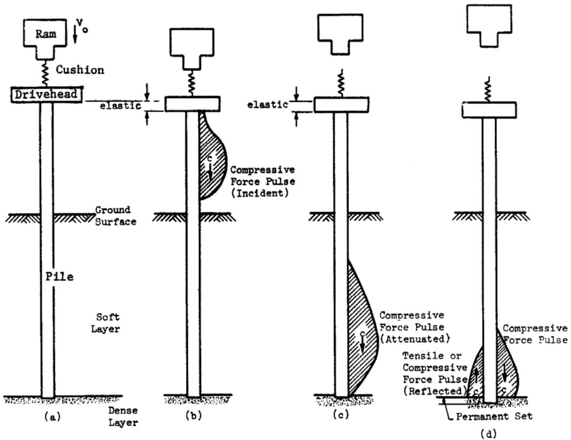
Figure 9-40. Hammer-pile-soil system.
