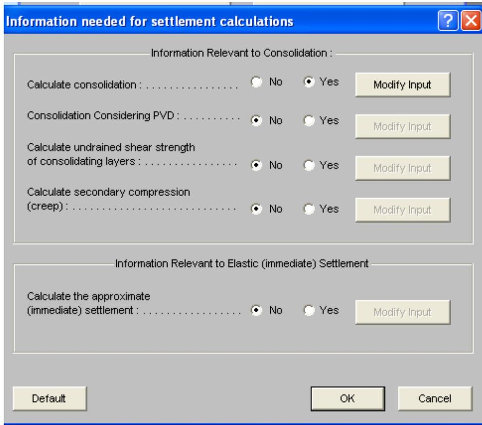
Figure E-6. Computation Manager Tab for defining the analysis case.
