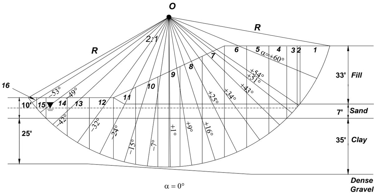
Figure A.5-5. Determination of  $\alpha$  – Angles corresponding to each vertical slice above assumed failure arc – East Abutment.
