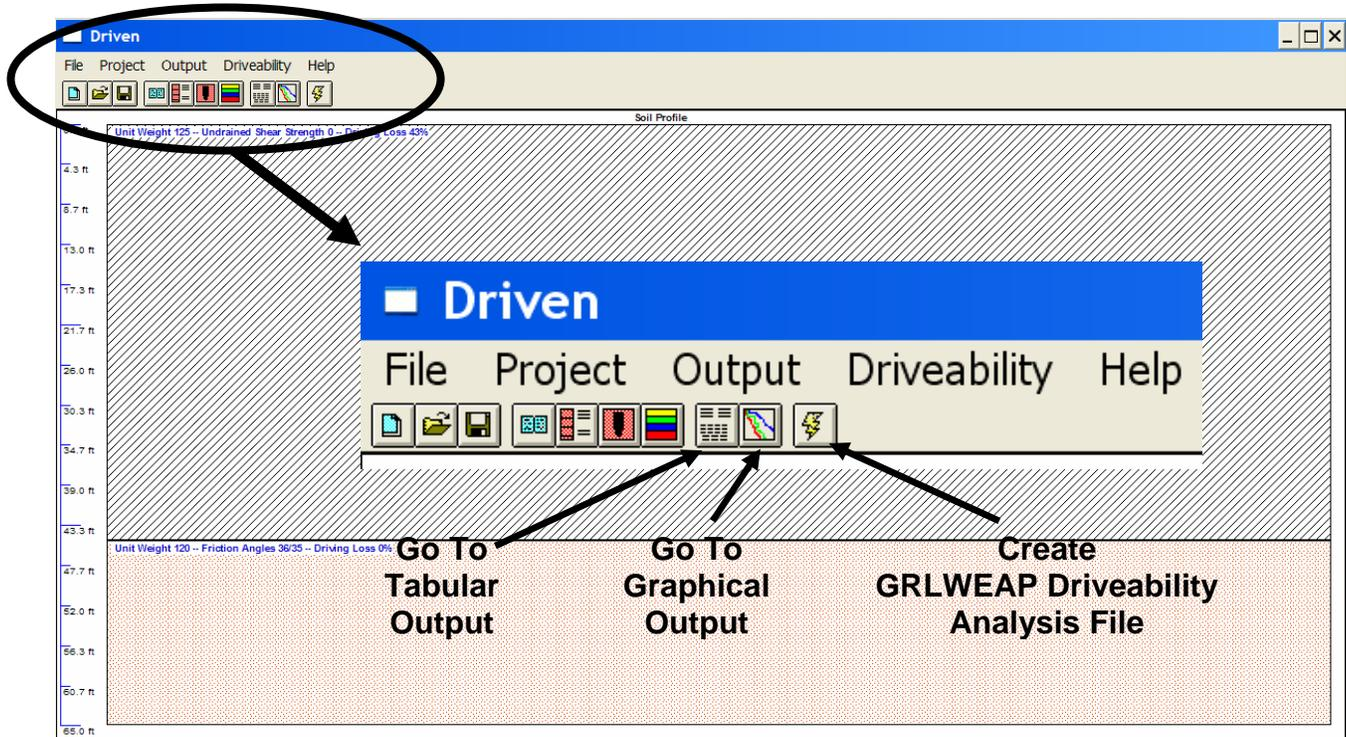
Figure 9-27. DRIVEN toolbar output and analysis options.
