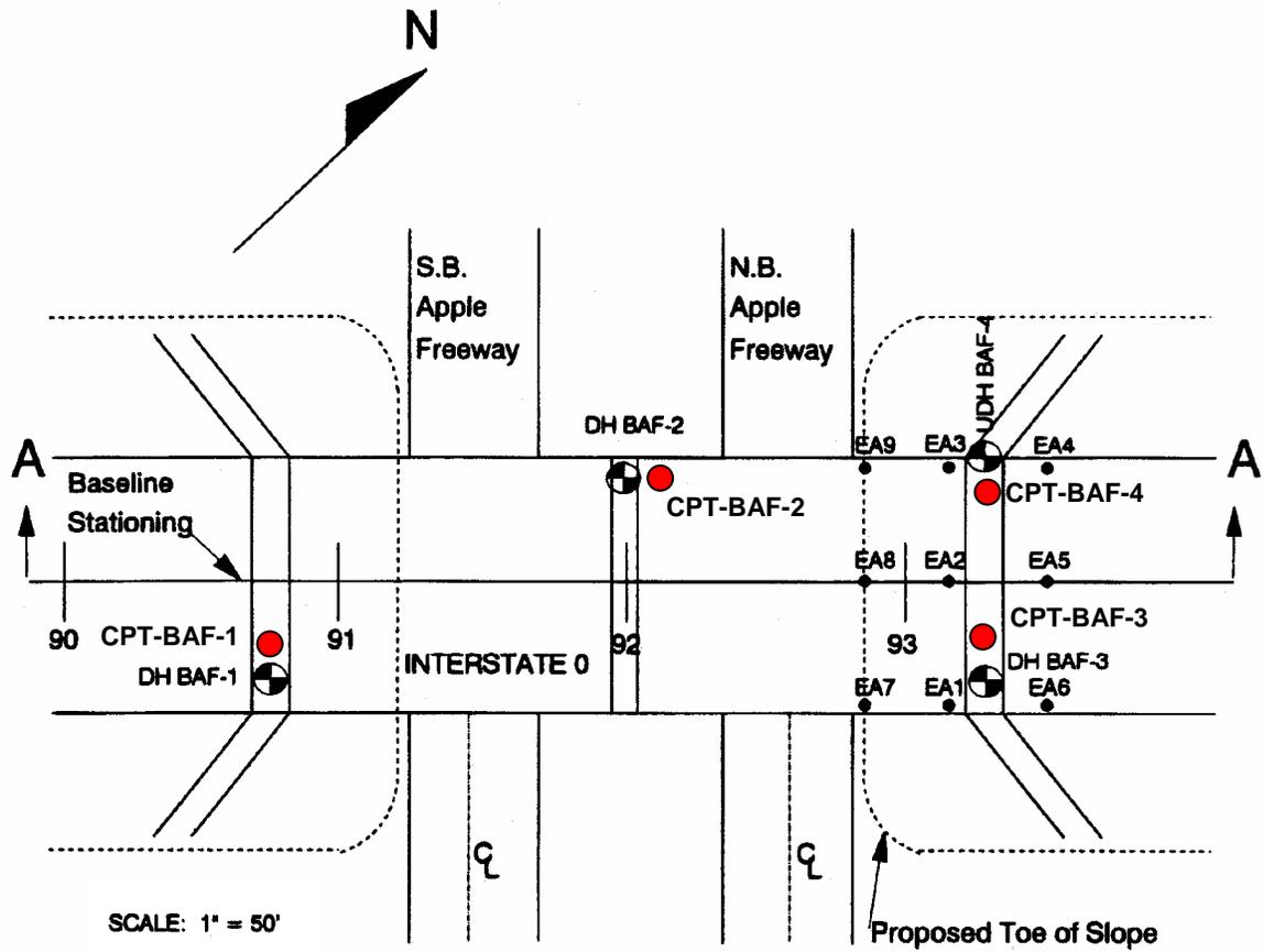
Figure A.2-4. Final field exploration layout.
