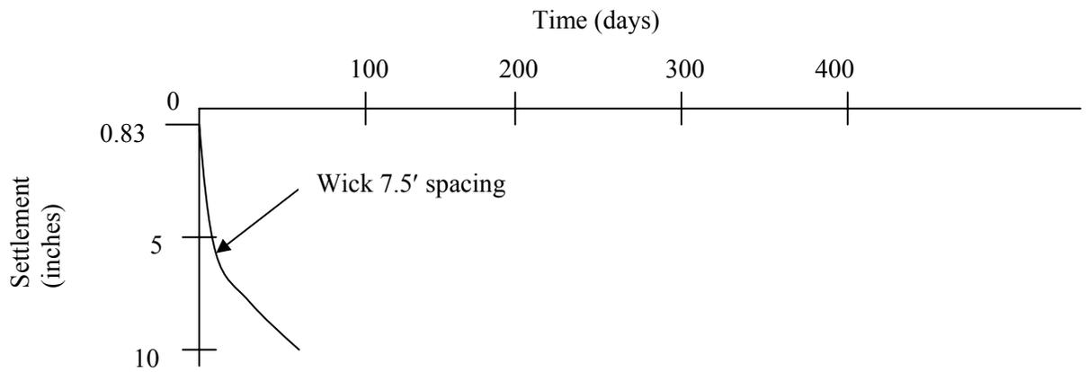
**Figure A.6-11. Time versus settlement after completion of embankment fill for wick drain treatment without surcharge.**
