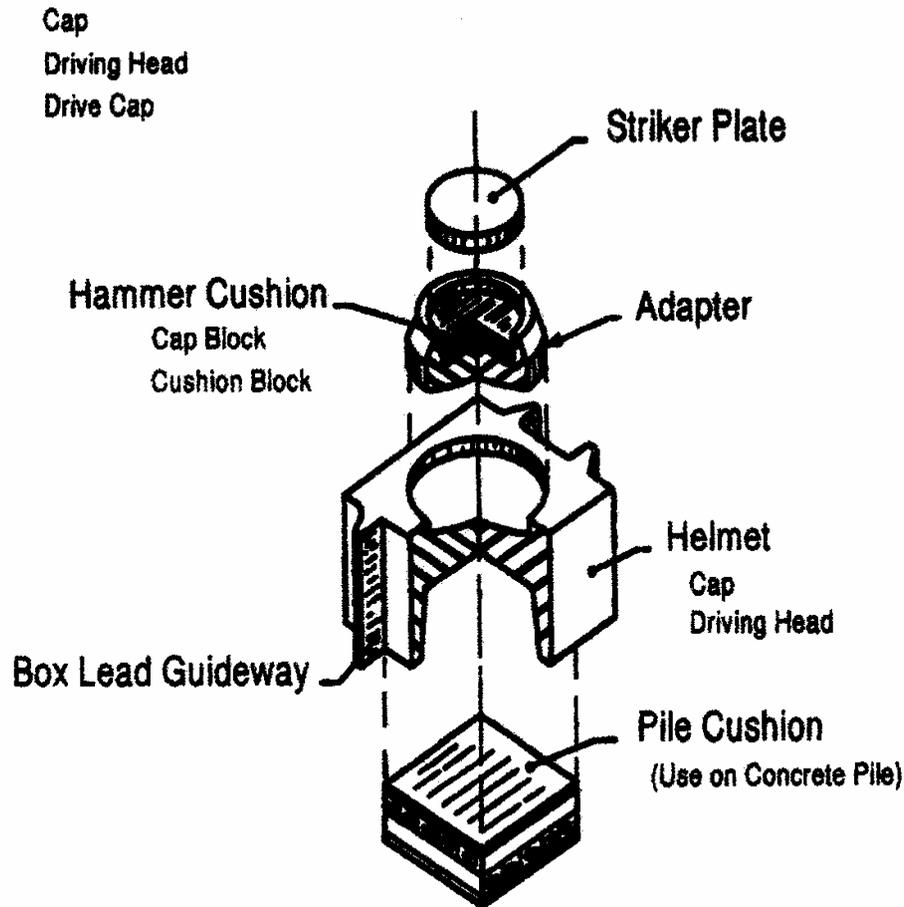
Note: The helmet shown is for nomenclature only. Various sizes and types are available to drive H, pipe, concrete (shown) and timber piles. A system of inserts or adapters is utilized up inside of the helmet to change from size to size and shape to shape.
