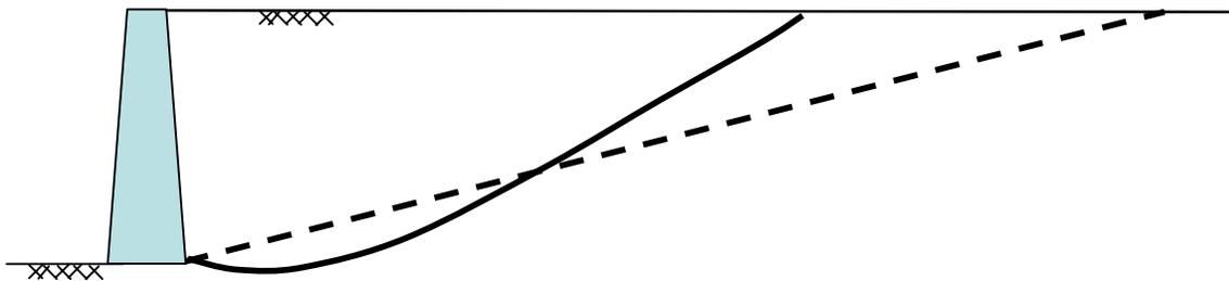
(b) Passive Case ( $\phi' = 30^\circ$ ,  $\delta = 30^\circ$ )
