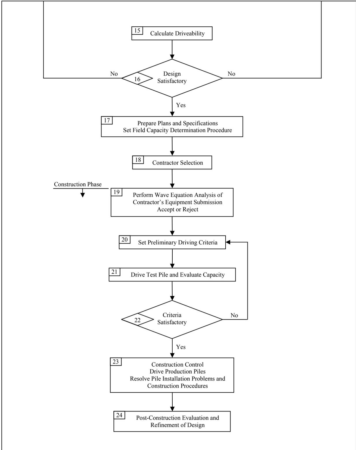
**Figure C-4. Driven pile design and construction process by LRFD (FHWA, 2006a)
