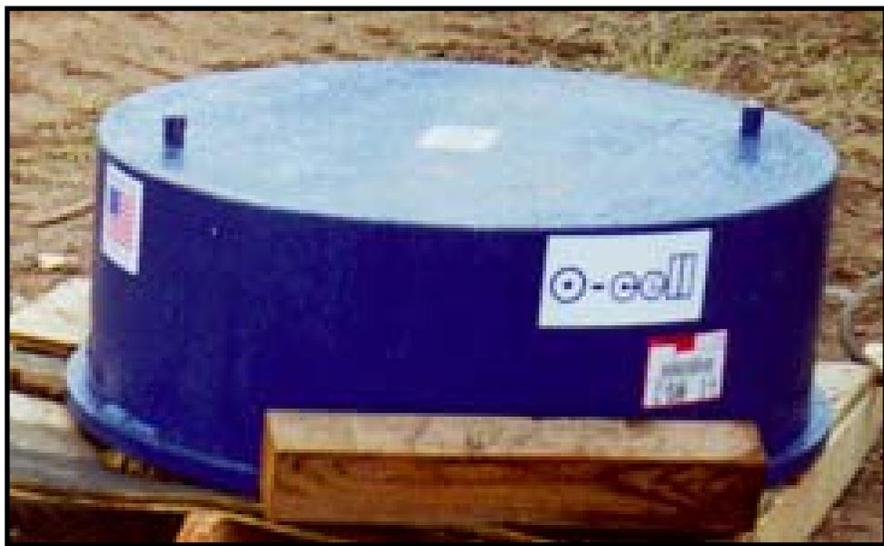
Figure 9-74. Photograph of an O-Cell<sup>®</sup>.
