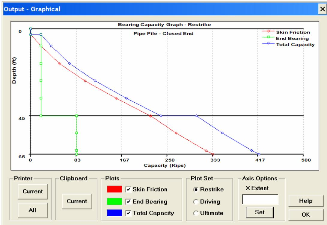
Figure 9-30. DRIVEN Output -Graphical screen for restrike.
